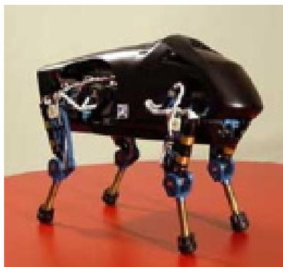
Figure 5.2: LittleDog manufactured by Boston Dynamics Inc.. The robot is used in the DARPA “Learning Locomotion” program with the goal to enable an unmanned vehicle to successfully traverse challenging terrains. One such terrain digitized from a real terrain patch is shown on Fig. 5.3. We use it as one of our test environments.
