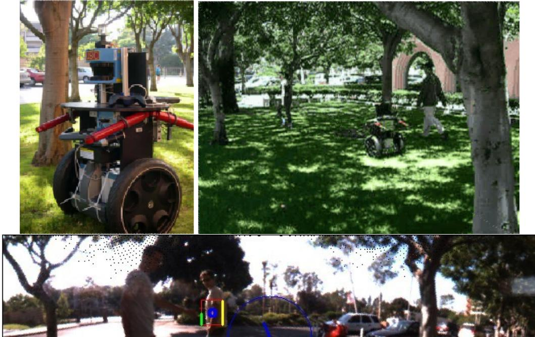
Figure 1.2: Segway RMP robot equipped with laser sensor, GPS, and omnidirectional camera (upper left). A typical scenario of following a fast moving person (upper right) and a view of the camera image of another scenario as the robot moves around the environment avoiding trees and tracking the correct person of interest
