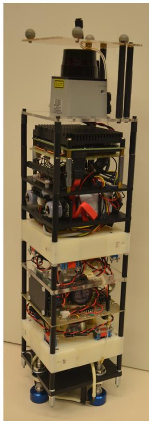
Fig. 2. The Cubesat engineering model with components related to autonomous proximity navigation.
