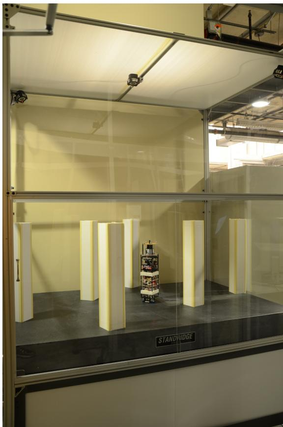
Fig. 1. The JHU Cubesat proximity navigation testbed.
